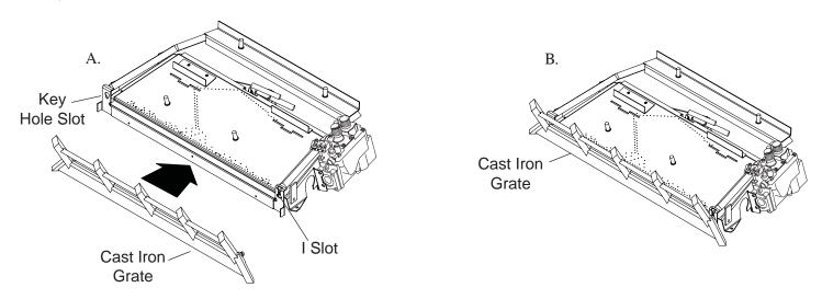
Figure 29 (a&b) - Installing Cast Iron Grate
